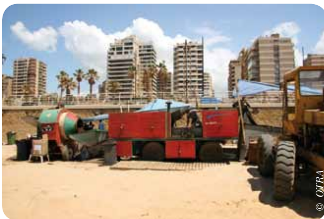
Mobile equipment for oil and sand separation in Beirut
