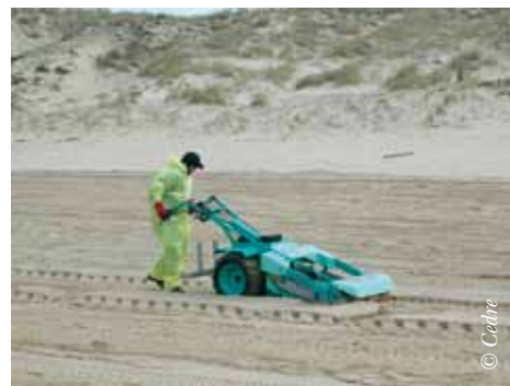
Mechanical selective sand screening
