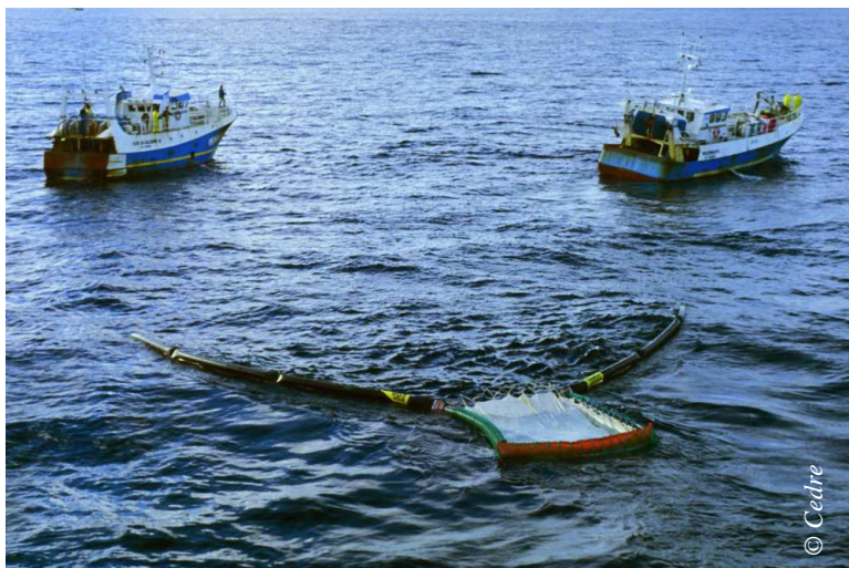
Dynamic recovery of oil using a specialised spill response trawl net
