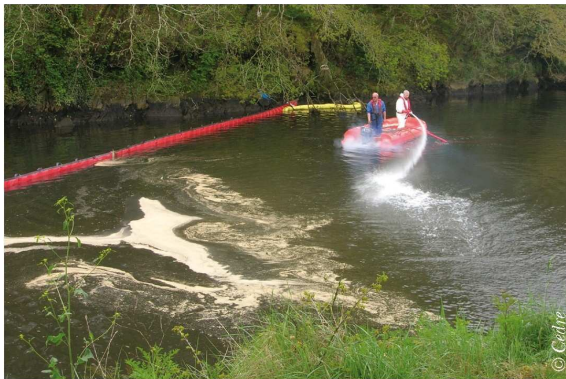
Slick of a light refined product: rapid spreading into a thin film
