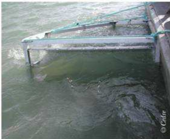
Specialised recovery equipment to facilitate the containment and manual recovery of the pollutant
