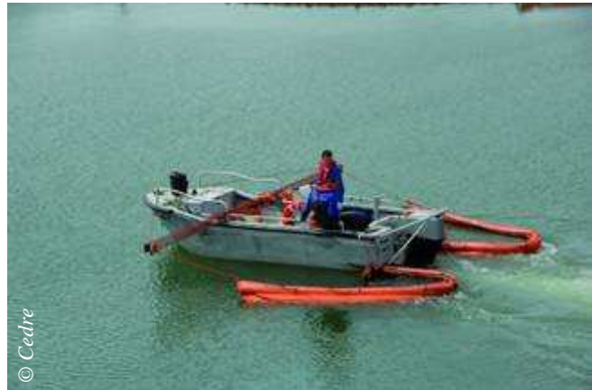
Dynamic recovery of a small spill using a sorbent boom with a ballasted skirt towed by a small boat
